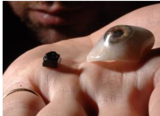
The prosthesis & the tiny camera it contains. (Credit: Eyeborgblog.com)
